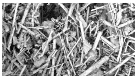
Figure 26 Lapinus CF + APP + TiO 2 600 °C (1112 °F)
