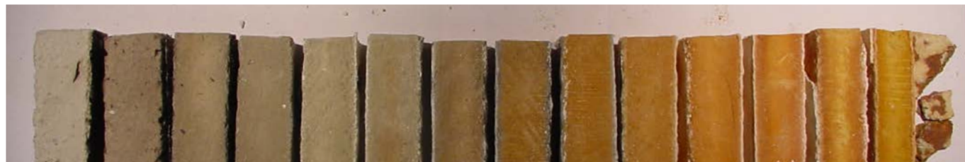
Figure 26 Lapinus CF + APP + TiO 2 600 °C (1112 °F)
