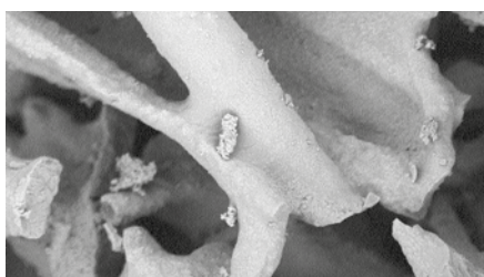
Figure 31 Lapinus MS + APP + TiO 2 1100 °C (2012 °F)
