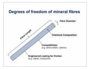
Figure 3: Mineral fibre characteristics
