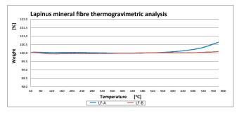
Figure 4: mineral fibre TGA: urves, existing versus new fibre grade
