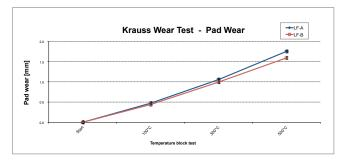
Figure 7: Pad wear comparison after SAE J2707 wear testing
